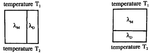
Fig. A1. The geometries with the minimum influence of the dispersed phase on the conductivity: (a) the minimum decrease for \lambda_D < \lambda_M ; (b) the minimum increase for \lambda_D > \lambda_M .
